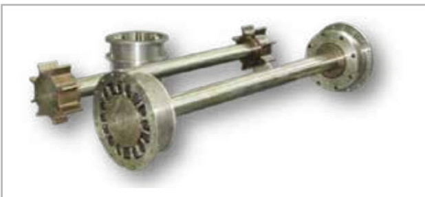
PCPM 40 Cardan Shaft Coupling for fan drive where motor was coupled to VFD for power saving to replace fluid coupling. DBSE was more than 2 mtrs. This was for a steel plant.
